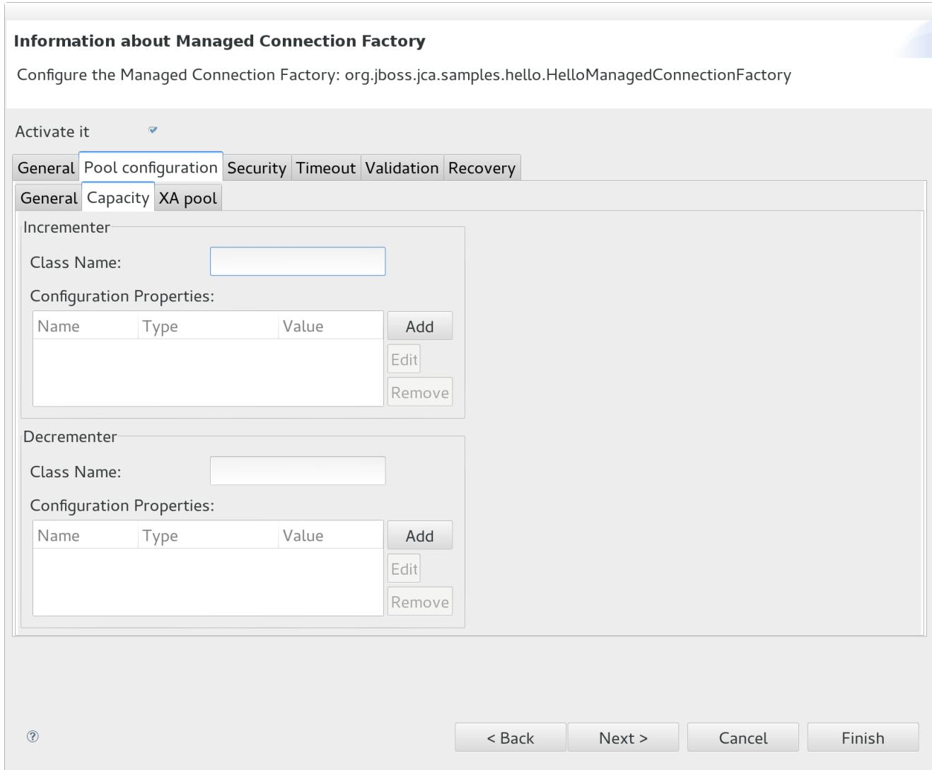
From IronJacamar 1.1 on, a capacity sub tab is added in 'pool configuration' tab to configure policy of connection pool
