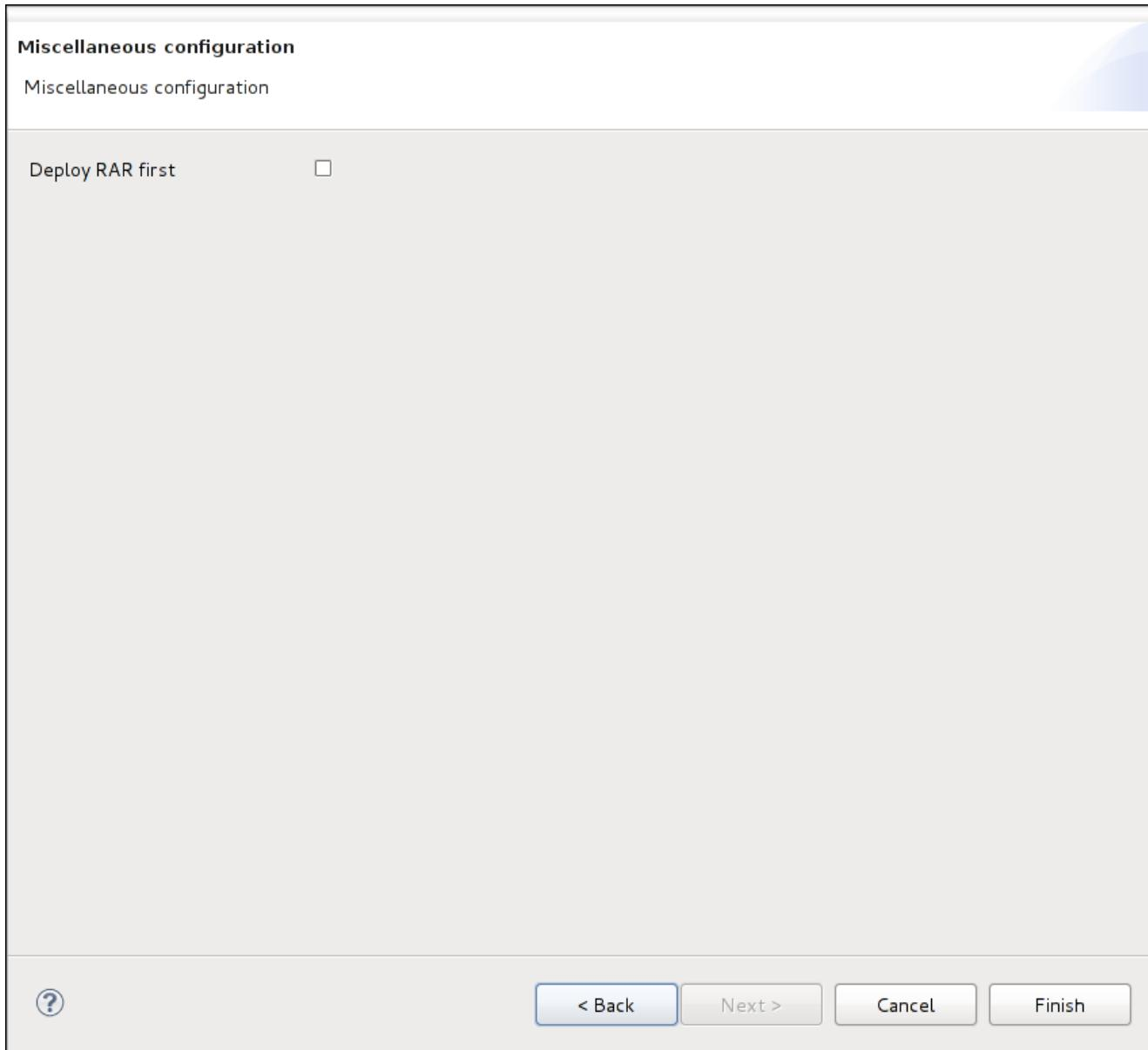
If the Deploy RAR first option is selected, the plugin will try to deploy the RAR file to the IronJacamar server first, then deploy the generated -ra.xml file.
